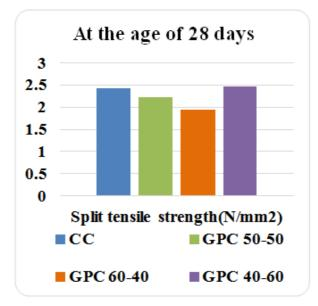
**Figure 2: Split Tensile Strength Comparative Chart**
